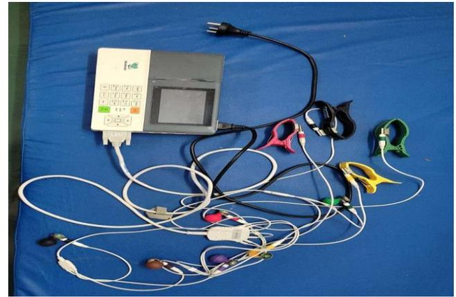
Figure 4 The portable ECG machine
